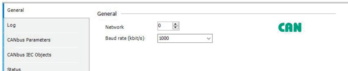
Then attach the CANopen\_Manager device to the CAN bus. The settings of this device depend on the following devices and must be adapted to them if necessary.
