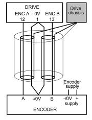
The drive will operate with 5-24V encoders. Provide the correct supply for the encoder. Do not use the 10V or 24V supply from the drive.
