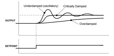
To set up the P gain, set the I gain to zero. Apply a step change in setpoint that is typical for the System, and observe the response. Increase the gain and repeat the test until the system becomes oscillatory. At this point, reduce the P gain until the oscillations disappear. This is the maximum value of P gain achievable.
