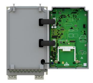
Remove and discard the Comms Option break-out feature in the control module housing by cutting the 7x bridges using suitable small side cutters.
