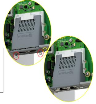
In the event that the Communication Interface Option Card needs to be removed, follow the installation process, but perform steps 7 and 8 in reverse.
