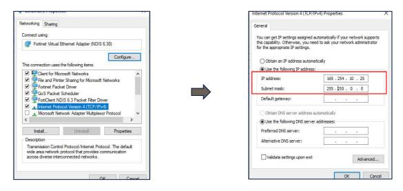
Alternatively, the IP address of the drive may be changed to suit the settings of the PC network adapter. The IP address of the drive can be configured using the DCT function, accessible from within DSE Lite by selecting Command -> Install AC15/AC20 Firmware.
