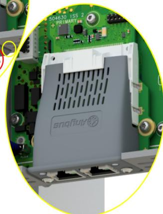
9. Now fully tighten the two T8 screws on the front facia of the Communication Interface Option Card.
