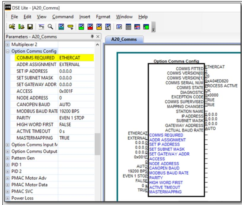
Alternatively, perform the steps described above by double clicking on the function block **Option comms config** to open parameters tab in the configuration interface.
