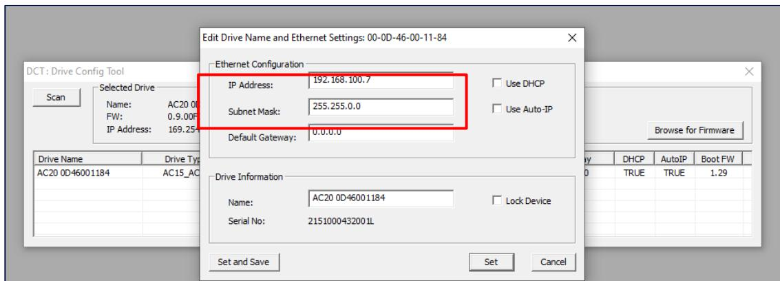
If the drive is not found by DSE lite, or a new drive is connected to the Ethernet port, a network scan must be performed again, as blow.
