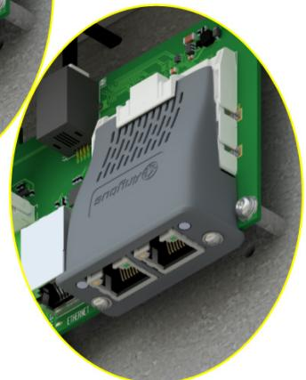
3. When the Comms Interface Option Card is fully engaged in the connector and its housing has hooked onto the edge of the PCB, fully tighten the two T8 screws on the front facia.
