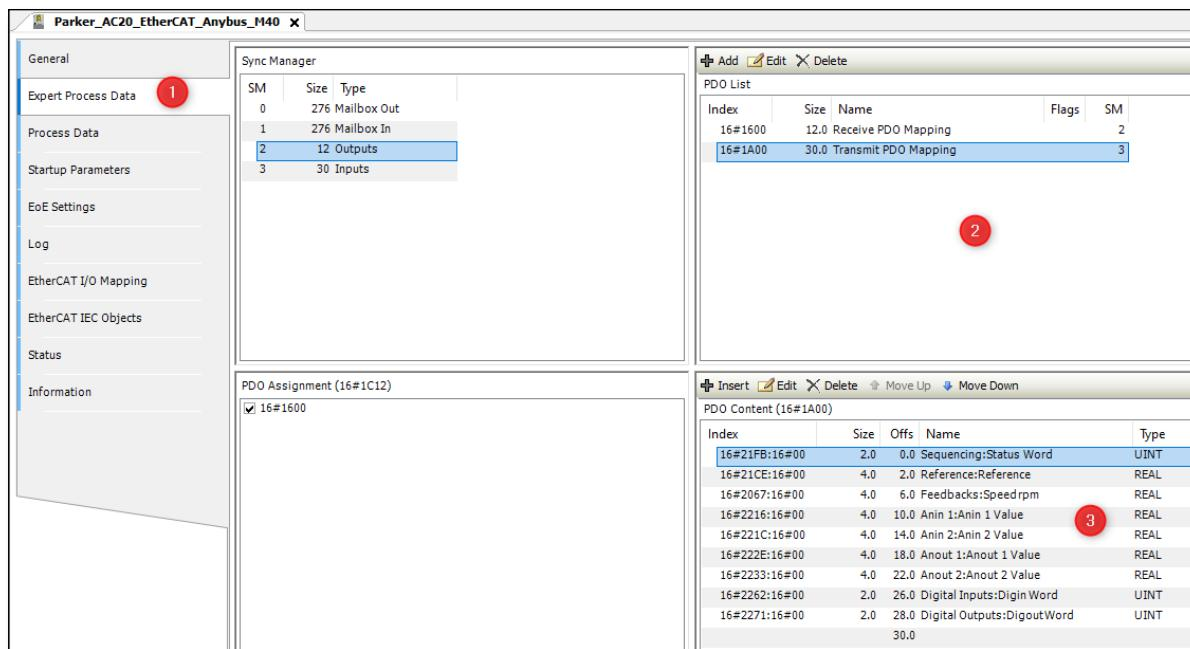
*Note: The AC20 Input/Output mapping table will be set to zero and will not have effect in this configuration.*
