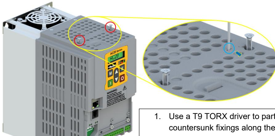
1. Use a T9 TORX driver to partially unscrew the two 3x12 countersunk fixings along the top of the product.
