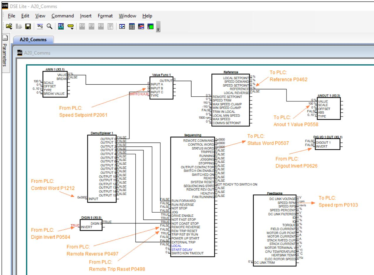
The data highlighted will be mapped into the AC20 process data mapping table in the example below.
