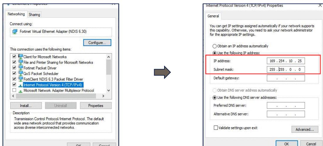
Alternatively, the IP address of the drive may be changed to suit the settings of the PC network adapter. The IP address of the drive can be configured using the DCT function, accessible from within DSE Lite by selecting Command -> Install AC15/AC20 Firmware.
