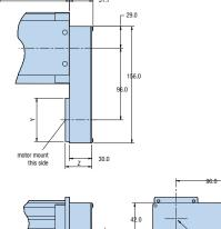
Parallel motor mounting is employed whenever a shorter overall unit length is needed. The motor is positioned along the sides or bottom of the table as designated by position A, B, or C. (No coupling required).
