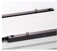
Two locating dowel pins shown in carriage
